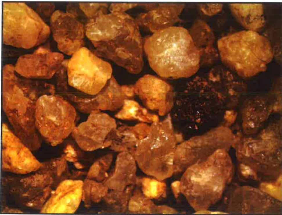
Figure 3: Digital image of coarse sieve fraction as recorded above. Note the secondary iron oxide in indents.
