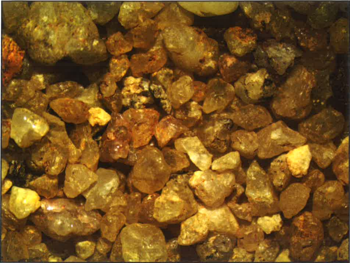
Figure 3: Digital image of coarse sieve fraction as recorded above. Note the secondary iron oxide in indents.
