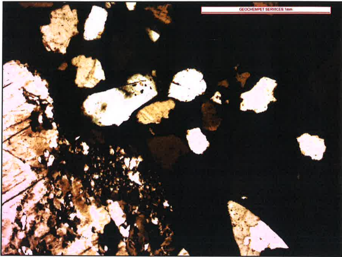
Figure 4: Micrograph of supplied sand sample, taken at low magnification under transmitted cross polarised light. Image shows a typical view of the sample, dominated by sub-angular to sub-rounded quartz showing a range of straining extinctions, along with minor lithic clasts of quartzite.
