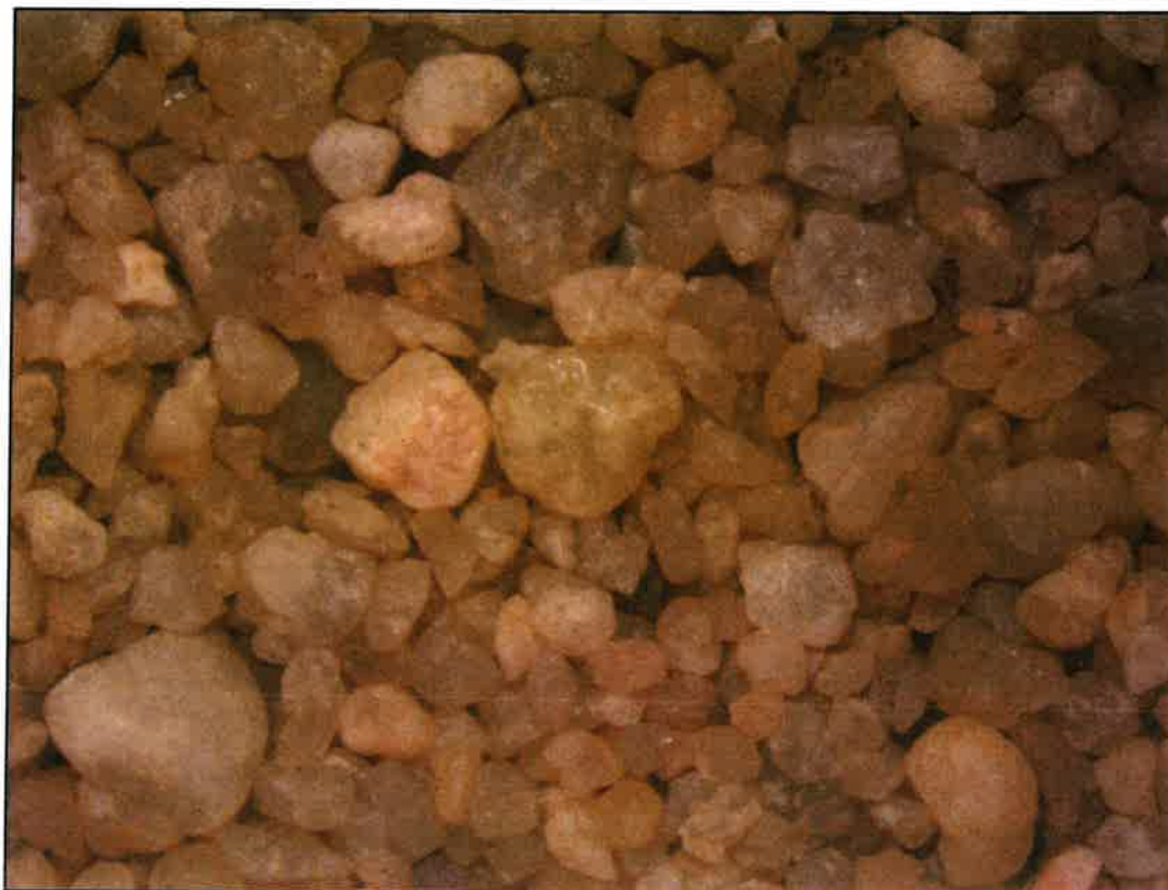
Figure 3: Digital image of coarse sieve fraction as recorded above; the view pictured is roughly 3.5 cm across.
