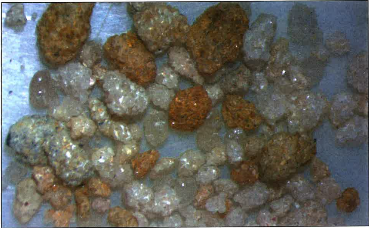
Figure 3: Magnified image of the coarse fraction, consisting of lithic sandstone fragments and minor quartzite and quartz grains.
